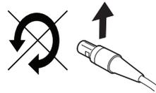
Pull the connector sleeve, not the cable itself to release the connector.
