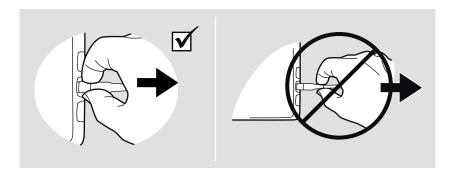
Pull the connector sleeve, not the cable itself or cable restrainer to release the connector.
