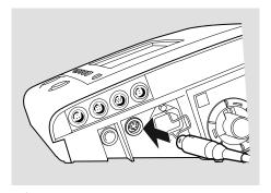
**2** Connect the other end of the cable to the DC source.
