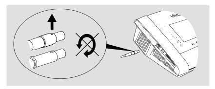
Insert the connector with the marking pointing upwards.
