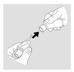
**5** Make sure to position the  $CO_2$ sensor with the LED pointing upwards.
