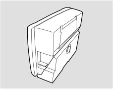
**6** Use the screw to secure the click-on battery by pressing it in and turn clockwise.
