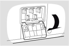
**3** Hold the Vivo 65 as shown in the picture, in order to target the click-on battery holders (marked with circles).
