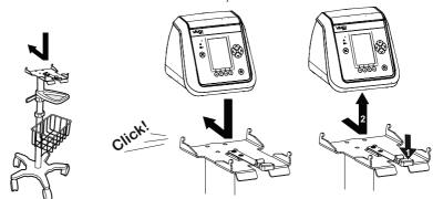
The bottom plate is mounted to the trolley using four
