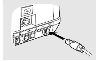
2 Make sure a clicking sound is heard to ensure the power supply is completely inserted.
