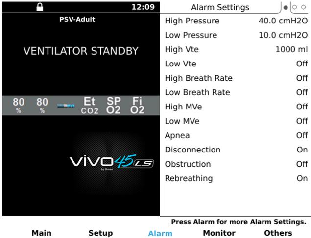
The Alarms section contains 3 pages: The two first are for viewing alarm settings and the third is for viewing the alarm and message history. Shift between the pages by pressing the Alarm button.
