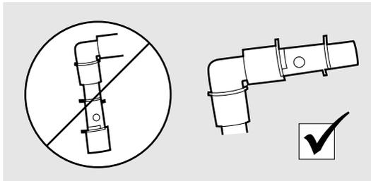
Do not place the airway adapter between the endotracheal tube and an elbow as this may allow patient secretions to block the adapter windows and result in incorrect operation.
