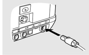
**2** Connect the other end of the cable to the DC source.
