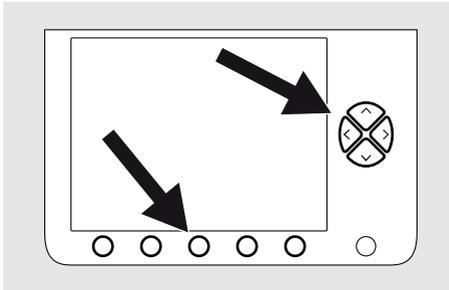
The navigation buttons are used to view the different sections defined above each navigation button. The same navigation button can also be used to view additional information in some sections, or it can be designated a temporary function while an event window is active.
