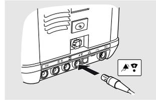
2 Test the connection by triggering an alarm on the ventilator and verify that the nurse call system activates.
