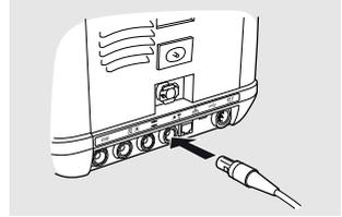
2 Make sure to insert the connector with the marking pointing upwards.
