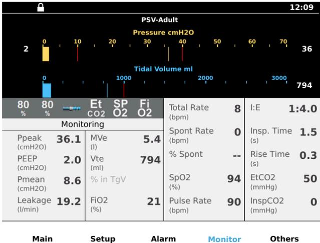
The monitoring page contains bar graphs for pressure and volume (or flow, during HFNT), and a field with measurement readings for the monitored values that are applicable for the treatment mode. See 5.3 Monitored Values in the Vivo 45 LS, page 56 for a description on the monitored values.
