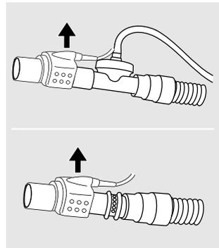
When installed, the ventilator automatically detects the sensor, also after powering off/on or after power failure.
