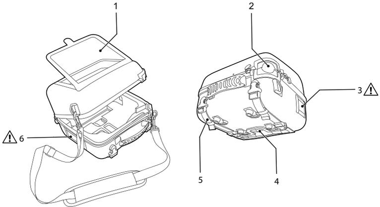
1. Transparent window, for accessing front panel and buttons
