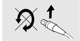
3 Pull the connector sleeve, not the cable itself or cable restrainer to release the connector.
