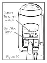
2. Press the Start/Stop Button a second time to stop treatment.
