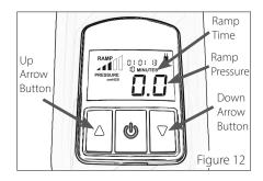
Ramp Time setting (this setting will be saved even when the *Z1* is not powered). The *Z1* will return to standby mode. To return to standby mode without saving the new setting, press and release the *Start/Stop Button* momentarily instead of holding it down.
